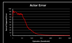
Figure 3: A simple (two-dimensional discrete grid) environment was setup to study the learning characteristics of the actor-critic model. The top graph shows the sum (over every possible state) of the squared error between the actor's policy and the optimal policy. The bottom graph shows the sum (over every possible state) of the squared error between the critic's value function and the optimal value function.
